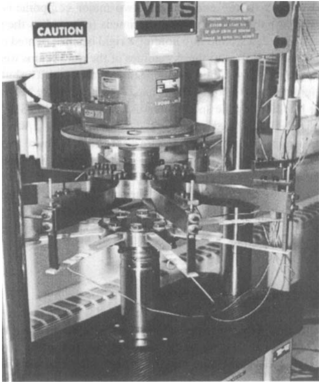
FIGURE 4 8 Specimens mounted on the “Octopus”-shaped fixture.
